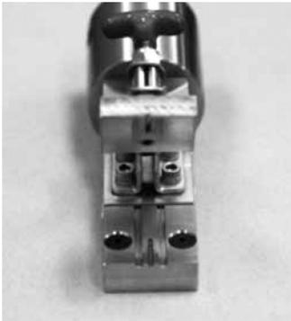
(b) Copper collar retention force: test set-up
